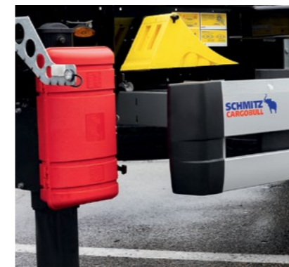
New side collision protection and fire extinguisher* on the support structure.
