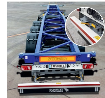
New design: fold-out underride guard for 45' containers is easier and safer to handle without loose parts that can get lost.
