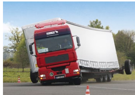
The bodies are certified in driving tests. First we test their durability with hydropulsers in the Schmitz Cargobull Validation Centre.
