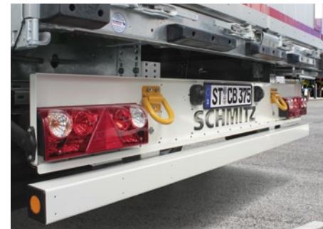
Stable during ferry transport: ferry lashings on the tail end secure the trailer during the crossing.
