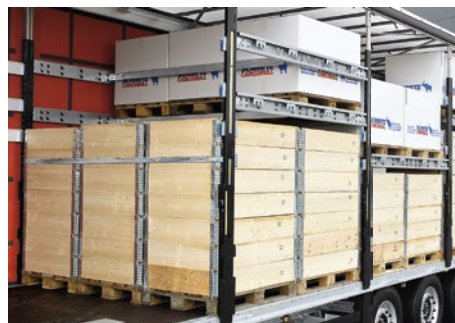
Cross beams between the stanchions or the side support beams allow the second level of freight to be securely loaded, e.g. in the HEAVY system.
