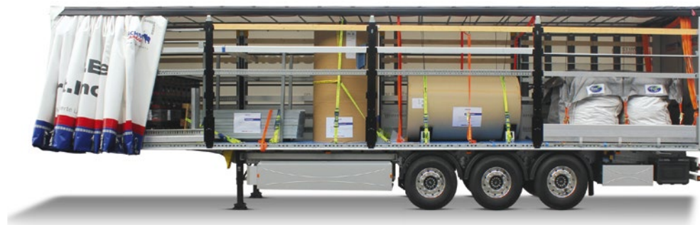
Sliding lashing system: lashing straps that pass over the roof can be positioned flexibly and quickly tightened by the driver without assistance.
