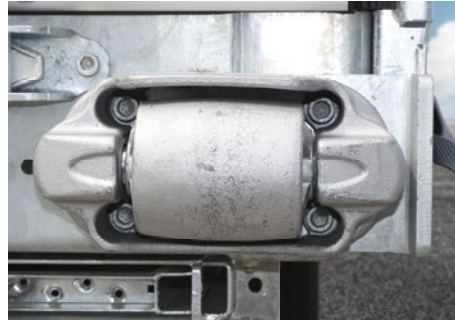
Compressible roller bumpers protect the rear wall frame when docking with the loading ramp.
