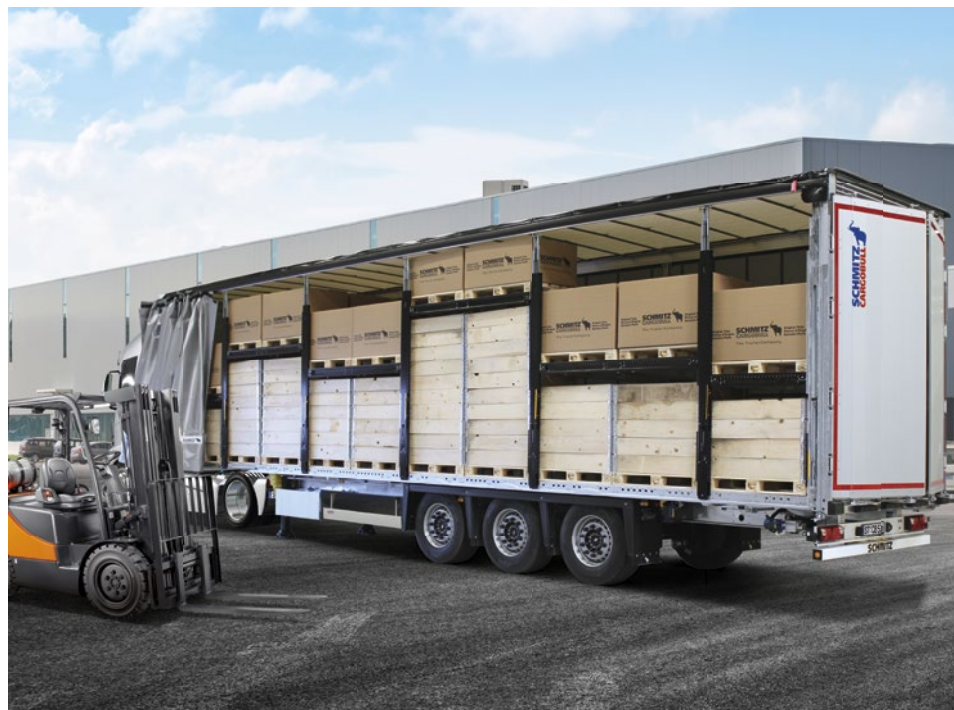
Variable utilisation of the load space with a total of 67 pallet spaces. Max. 3,050 mm usable internal height with the S.CS MEGA.
