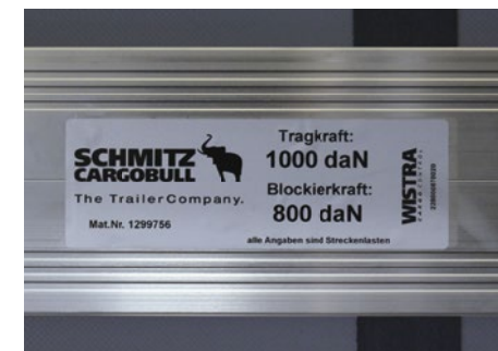
The cross beams provide a payload of 1,000 Nm and can also be used for load securing with 800 daN. (LIGHT system)
