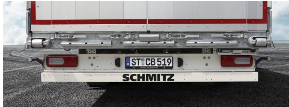
Modular design of ramp package provides for ease of replacement in the event of damage.
