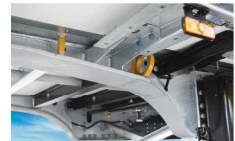
Special lashing points are provided on the I-beam and frame to secure the trailer to the ferry, even in rough conditions.
