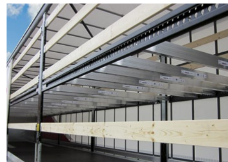
The double-decker system is quickly assembled and the LIGHT version can also be adapted to the S.CS UNIVERSAL.
