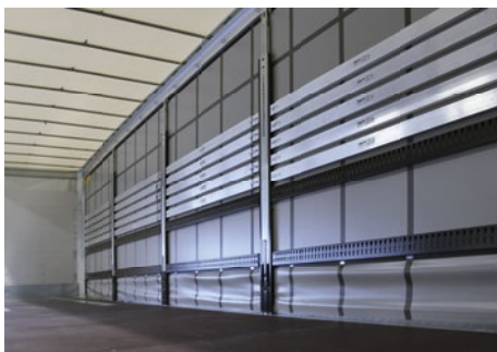
When parked, the double-decker floor can be stored between the stanchions or in front of the front wall.
