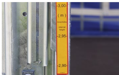
Three heights in the S.CS MEGA – the interior height is adjusted in 50 mm increments by the use of perforated rails.
