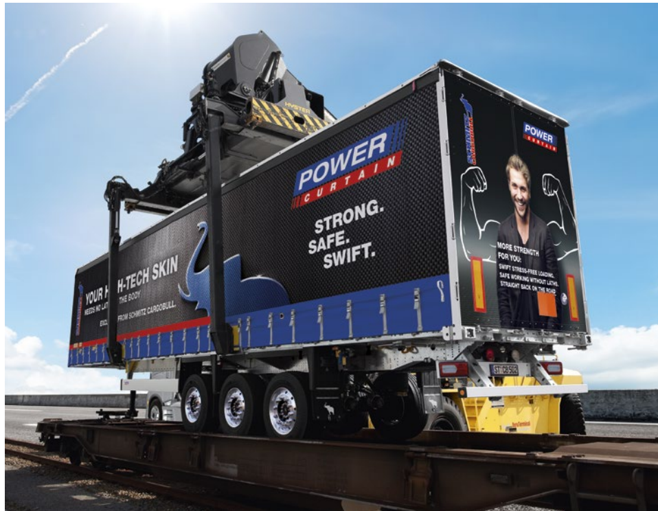
The trailer can be loaded unaccompanied onto rail vehicles for long-distance journeys: part units in multimodal transport are an economical alternative, for instance on transalpine journeys, as the tractor unit can be used elsewhere during this time.
