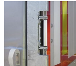
Rear corner supports have integrated ram protection over the entire height of the hinges.
