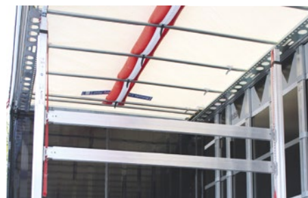
Partial loads can be flexibly secured using locking bars and cross beams.
