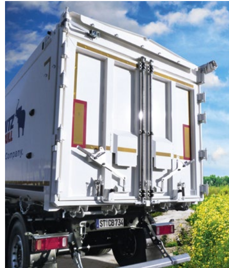
Combi-door: controlled unloading through the grain slider, tipping by the pendulum tailgate, loading through open doors.
