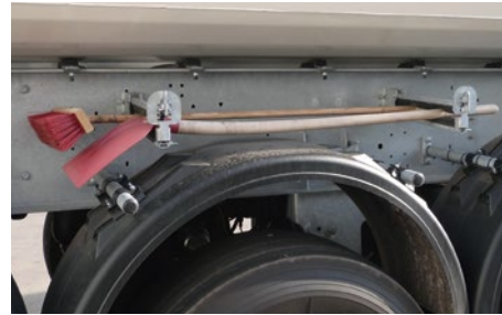
The brush and shovel are easily accessible and rapidly stowed.
