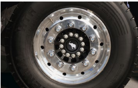
Lightweight aluminium rims for weight reduction and a high-quality appearance.
