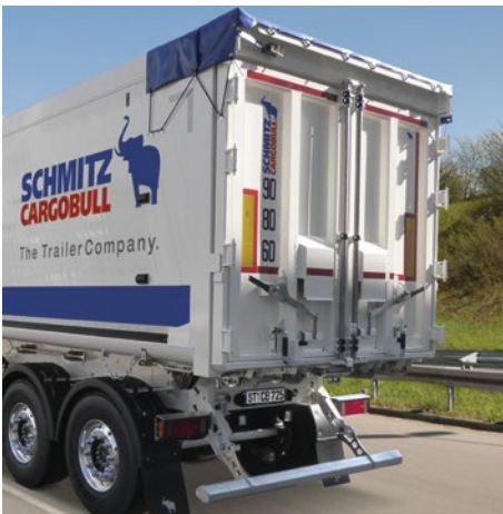
Combi-door with closed pendulum frame and wing door.
