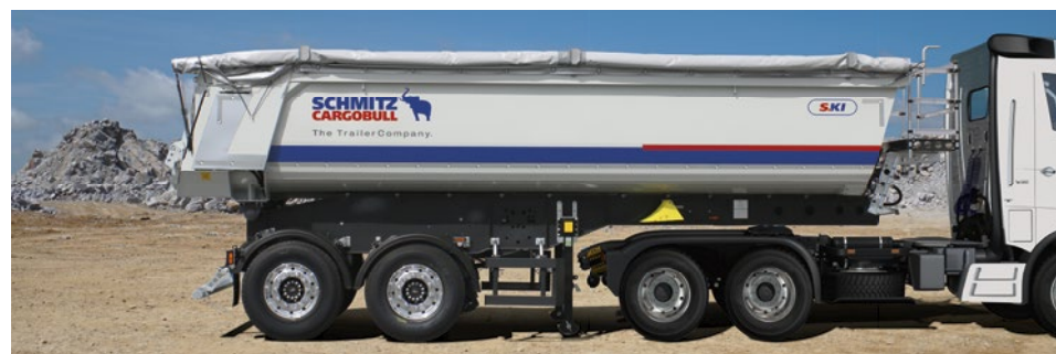
The low centre of gravity of the body optimises tipping stability. The tilt angle assistant issues a warning in the event of excessive sideways tilting.*
