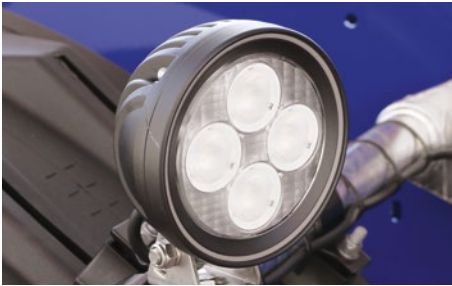
Additional reversing lights with LED technology.*
