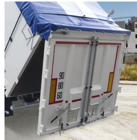
The central tube in the roller tarpaulin makes the covering more stable.
