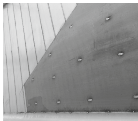
Wear plates optimise the durability of the rear part of the aluminium box body**.
