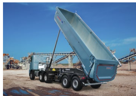
The low centre of gravity of the body optimises tipping stability. The tilt angle assistant issues a warning in the event of excessive sideways tilting.*
