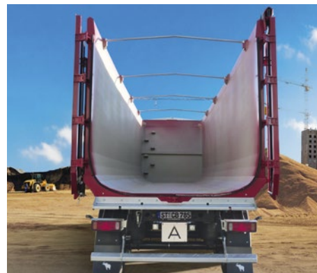
Double wing door open and bow for the roller tarpaulin.
