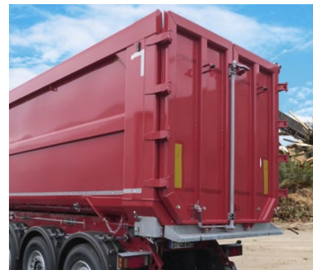
The double wing door with short chute makes the body very accessible.
