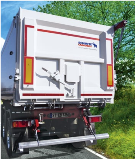
External pendulum tailgate with rubber seals on all sides, grain slider, four-hook locking and side clamping locks.
