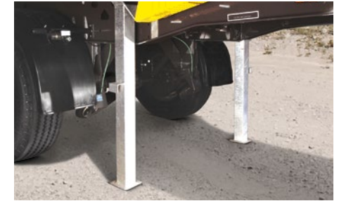
Lightweight detachable stabilisers are the right solution for permanent tractor-trailer units, the trailers of which are rarely disconnected.
