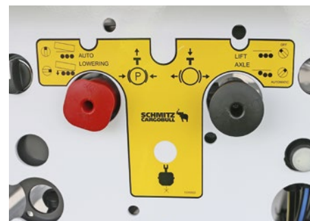
The automatic lowering function provides greater stability when tipping and can be deactivated if necessary.
