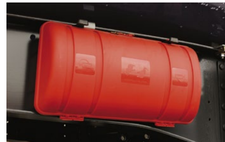
The fire extinguisher on the chassis is quickly accessible in the event of an emergency.
