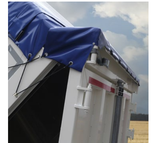
The body can be emptied using the pendulum function when the roller tarpaulin is closed.
