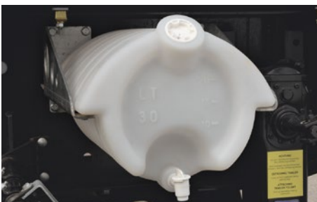
Water tank for 30 litres on the I-beam.
