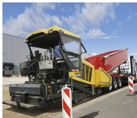
The folding underride guard provides greater clearance when tipping the asphalt into the road paver.
