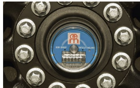
The odometer mounted on the wheel hub provides information about the tipper semi-trailer's mileage (km).
