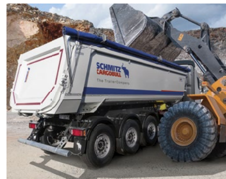
The flat base of the rounded steel body provides a lower loading edge, whilst retaining the same volume.
