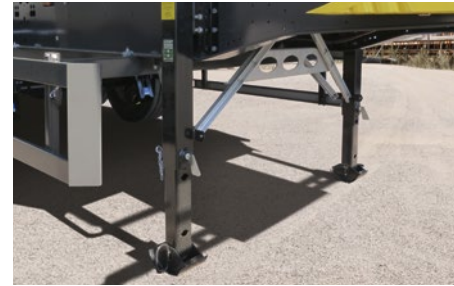
The steel drop supports are secured with locking pins – a weight-saving solution.
