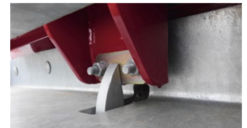
Locked: the hooks on the safety locks lock the doors of the tipper body.
