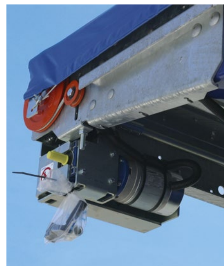
The bevel gear and the drive for the sliding roof are protected beneath the protective canopy of the front wall.
