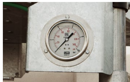
Overloading protection: the loading pressure gauge shows the air bellows pressure.
