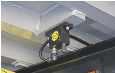
Compressed air roller vibrator for even fast-flowing bulk materials and shorter unloading times.
