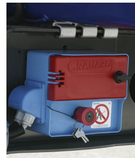
The control panel for the electric sliding tarpaulin is fitted to the longitudinal beam.
