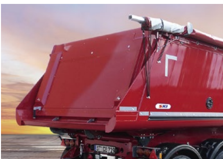
Internal pendulum tailgate with chute.
