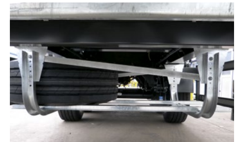
Spare wheel basket under the chassis, in front of the axle unit.
