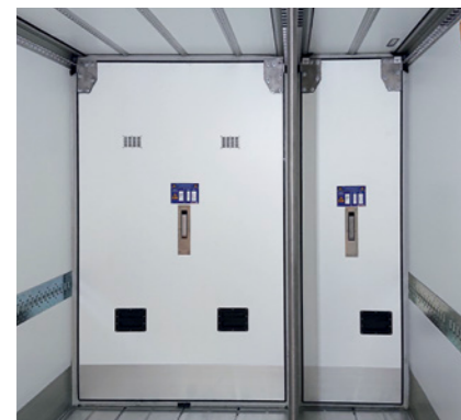
Sliding partition wall made of highly insulating FERROPLAST®: Fast, variable MultiTemp partitioning; optionally available for 1/3 and 2/3 partitioning or as a continuous wall.
