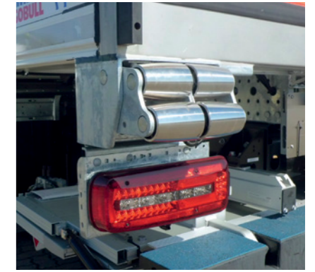
Dynamic Ramp Protection (DRP) and a double rubber strip protect the rear end when approaching the ramp.
