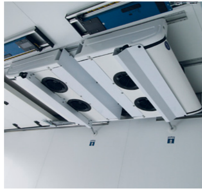
Ceiling-mounted auxiliary evaporator for MultiTemp versions and trailers in through-loading trains.
