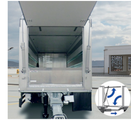
Transition in the through-loading train: End wall flap for trailer Z.KO is folded up as weather protection, folded up and distance adjusted with pneumatically locked, extendable drawbar.*
