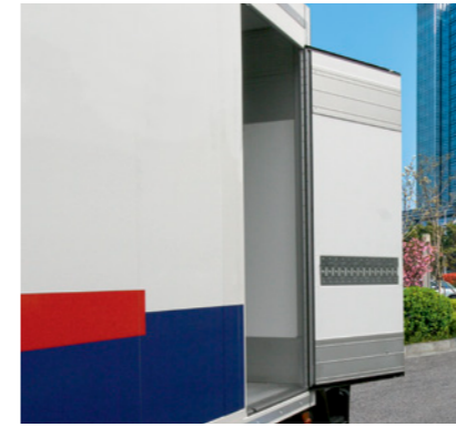
Side door allows for partial unloading and separate access to individual MultiTemp cooling zones.
