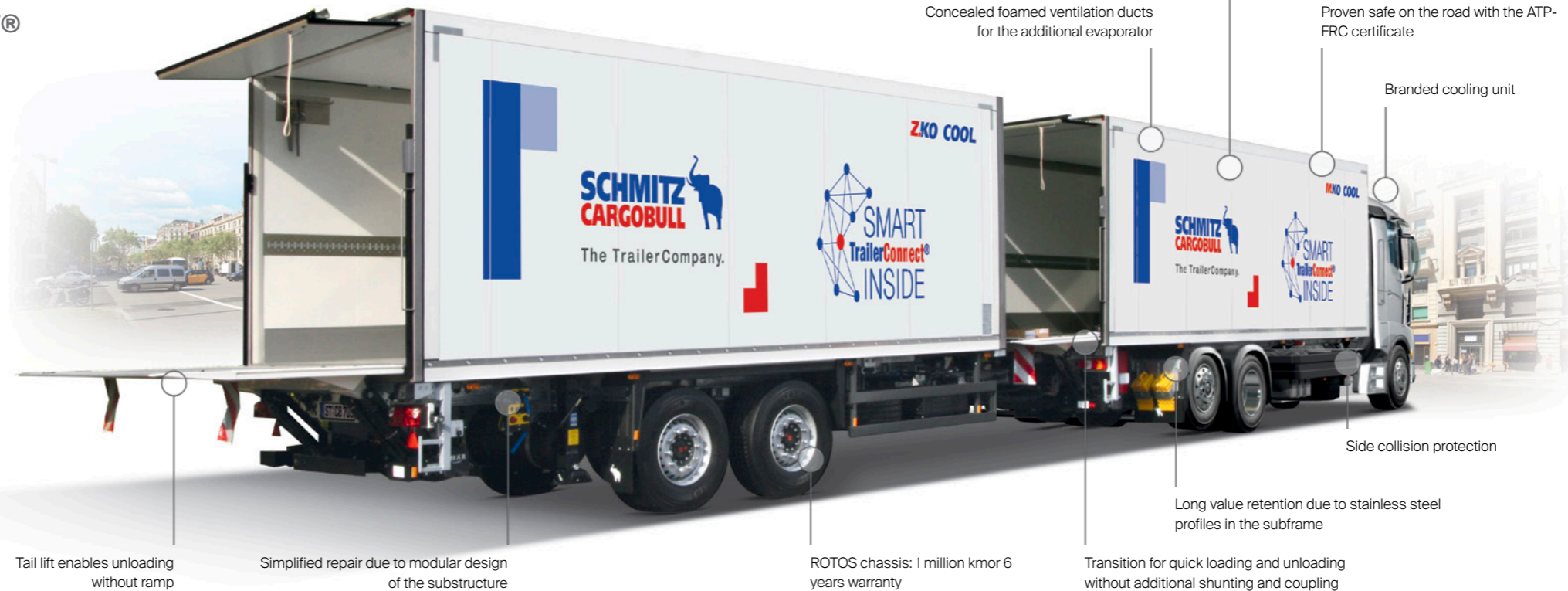
FERROPLAST® structure with improved insulation
