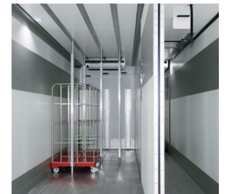
Airline rails in the ceiling and floor simplify load securing with vertical telescopic beams.
