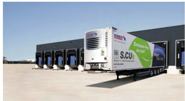
Fully electric refrigerated box body with electric transport cooling unit for zero-emission, quiet deliveries to supermarkets
