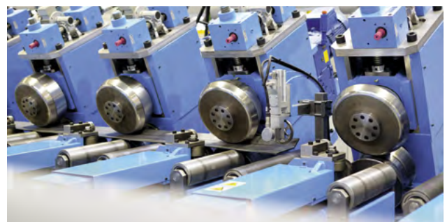
L-beam production: The galvanised longitudinal members for curtainsiders and dry freighters are cold-formed without any welding.
