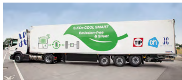
Fully electric S.KOe COOL SMART refrigerated box bodies: The electric trailer axle recovers energy and reduces the cooling unit battery's charging time.
