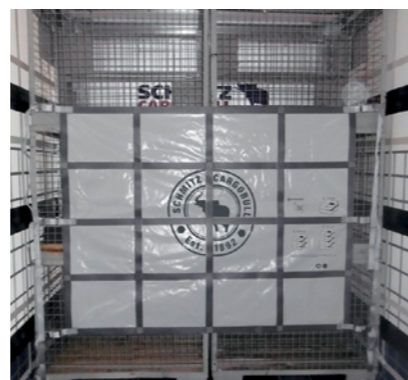
Rear load-securing for partial loads with the integrated tarpaulin loops e.g. for tension belts or securing tarpaulins. In three rows one above the other, the loops have a securing force of up to 7,500 daN for partial loads (2,500 daN per row).
