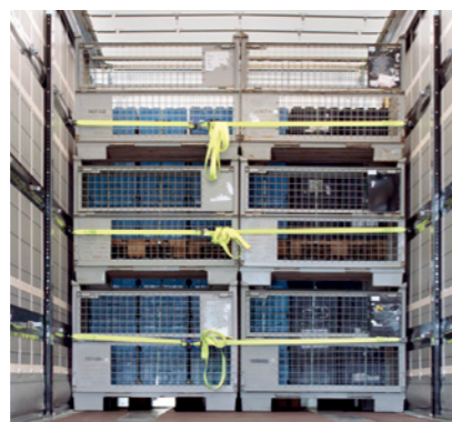
Rear load-securing for partial loads with the integrated tarpaulin loops e.g. for tension belts or securing tarpaulins. In three rows one above the other, the loops have a securing force of up to 7,500 daN for partial loads (2,500 daN per row).
