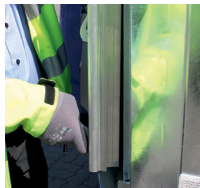
Hook strip on the end wall for hooking the tarpaulin into the reinforced edge, resulting in a higher tensioning force.
