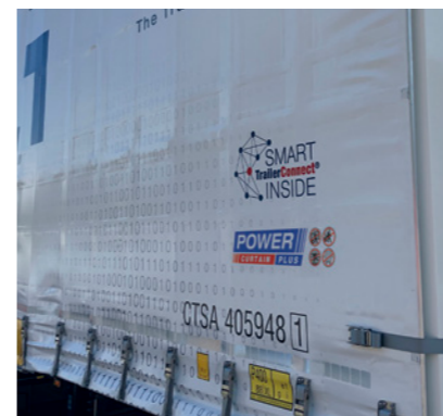
"Board-hard sidewall" for all non-palletised goods that place a heavy load on the side tarpaulin. Vertical supporting bars** prevent bulging.
