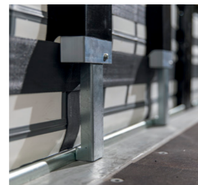
Fixed at the bottom - Slide-out metal profiles use the continuous pallet stop of the outer frame to keep the supporting bars** stable at the bottom.
