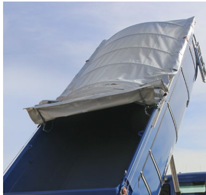
Electric sliding tarpaulin: temperature-resistant, and can be operated easily and quickly from the ground.
