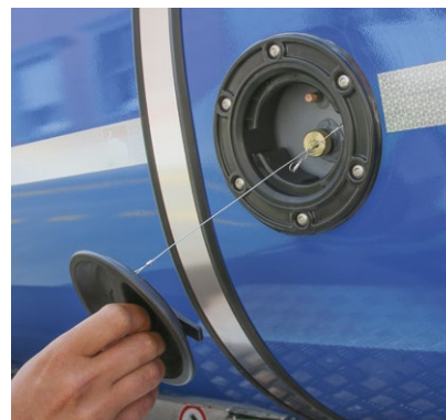
Future-proof: optional access points for manual, direct temperature measurement and preparation for the installation of electronic measuring technology.
