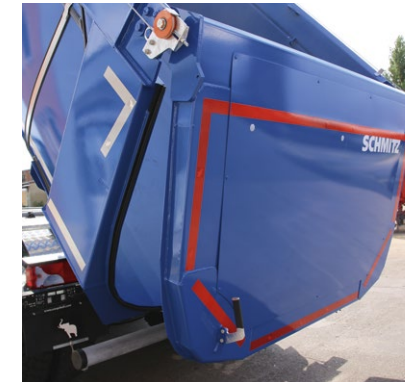
External pendulum tailgate with rubber seal around the lip.
