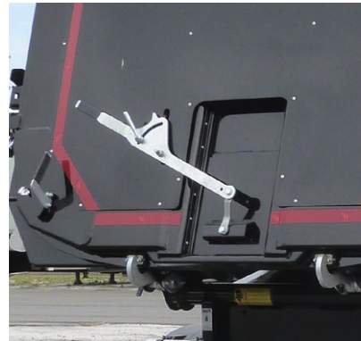
Central slider: with an external pendulum tailgate for controlled unloading (option).
