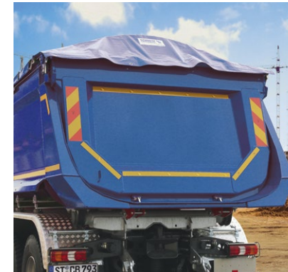
Internal pendulum tailgate with chute for centred unloading.
