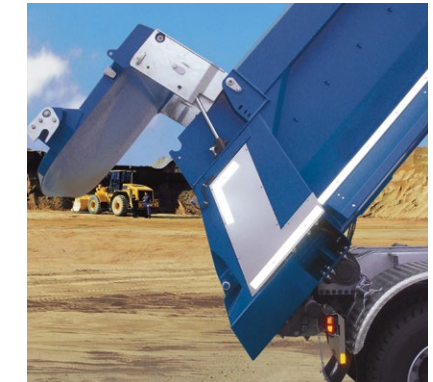
Hydraulic tailgate: ideal for abrasive, coarse bulk materials and controlled unloading.
