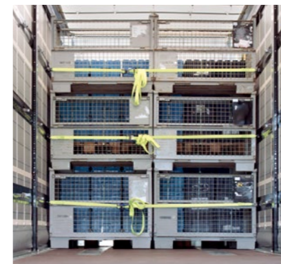
Rear load securing with stitched-ontarpaulin loops for tensioning belts or safety tarpaulins. Arranged in three rows above each other, the loops have a securing force of up to 7,500 daN with partial loads (2,500 daN per row).
