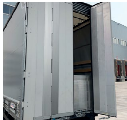
Sectioned portal on the bulkhead: the four-wing door enables the portal to be opened in the narrow space between the truck body and the trailer.
